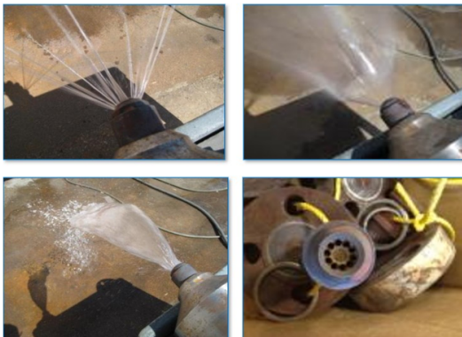
Figure 4: A loss-of-effectiveness actuator fault can manifest through various forms of nozzle damage, each degrading spray performance. Examples include plugging (top left), out-of-spec spray patterns (top right), broken nozzles (lower left), and completely detached or blown-off nozzle tips (lower right) [13].
