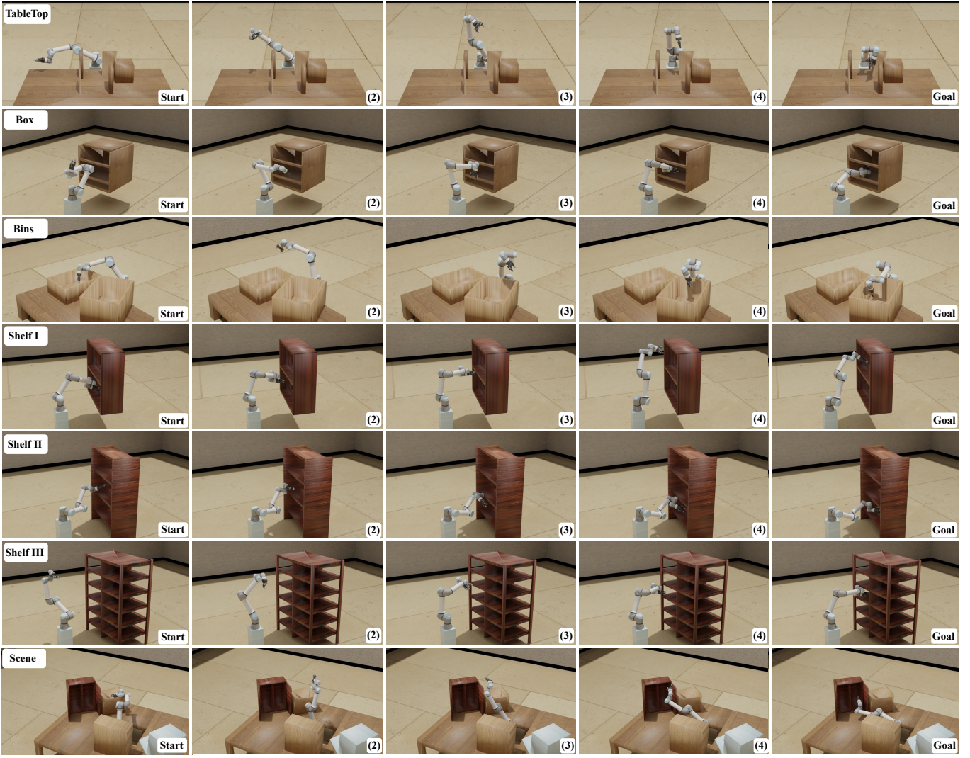
Fig. 8: Simulation evaluation: \pi NetsFusion planning in held-out planning task and an out-of-distribution Scene (bottom row) generated by MotionGeneralizer with planning time of 0.2 \sim 0.3 seconds. The path profile from start configuration to the goal configuration is demonstrated through frames 2-4.
