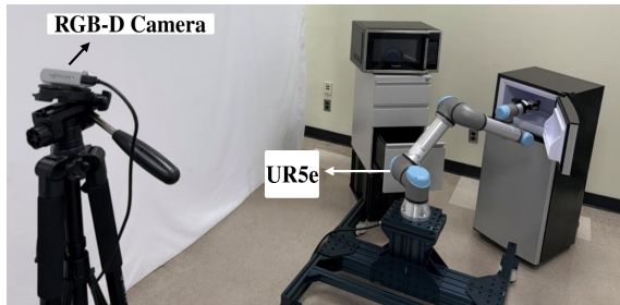
Fig. 11: Experimental Setup for real-world deployment of M \pi NetsFusion on UR5e robotic manipulator. The calibrated RGB-D camera is an Intel RealSense D435i used to capture workspace observations.
