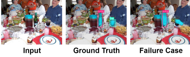
Figure S3. Failure case on the IIT-Heat dataset. Missing detections in real-world cluttered scenes lead to incomplete cues for the affordance learning branch.
