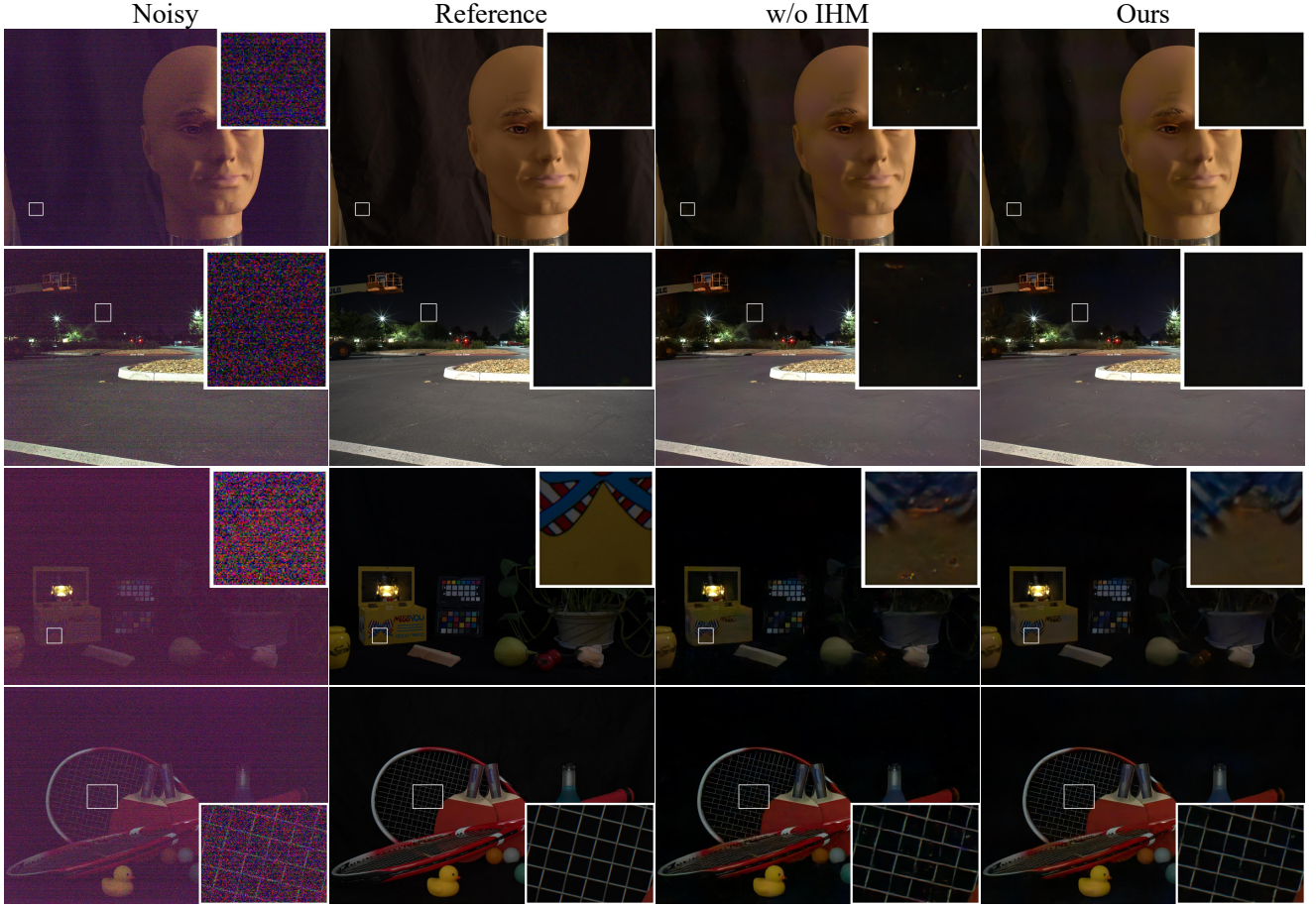
Figure 11: Ablation study on the iterative histogram matching (IHM). Without IHM, noticeable white spots appear in the denoised outputs due to saturated pixels in the noisy inputs. With our full method, this issue is effectively mitigated. The first two examples are from the SID test set while the third and forth are from the ELD test set. Best viewed zoomed in.
