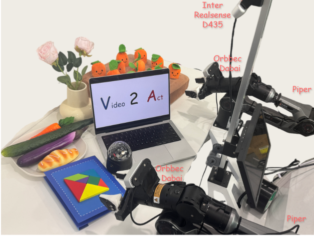
Figure 8. Real-world robot setup and experimental assets. We utilize the Agilex Cobot Magic platform with four 6-DoF Agilex Piper robotic arms, equipped with an Intel RealSense D435 head camera and two Orbbec Dabai wrist cameras, along with the object assets used across all real-world tasks.
