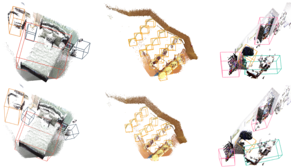
Figure 5. Qualitative prediction results on the SUN RGB-D. The first row displays the ground-truth data, while the second row presents the detection results from our GraphFusion3D.
