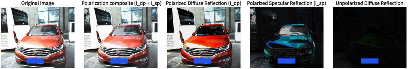
Fig. 3: Separation results of specular and diffuse components based on polarized images.
