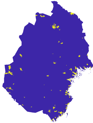
Figure 9: Cellular Coverage Map of the Arctic Region of Sweden for a data rate of 30 Mbit/s and low sensitivity for 2019 created using (4).
