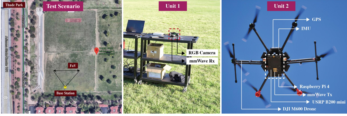
Fig. 3: Real-world multimodal data acquisition and testing setup, as shown in [13]. The system includes a BS (Unit 1) equipped with an RGB camera and mmWave receiver, and a UAV (Unit 2) carrying GPS, IMU, and mmWave transmitter.
