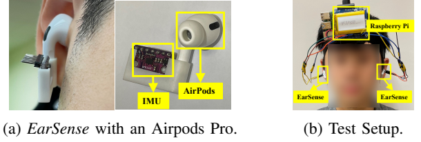
Fig. 2: EarSense is an open-sourced data collector attachable to commercial earables for vibration sensing.
