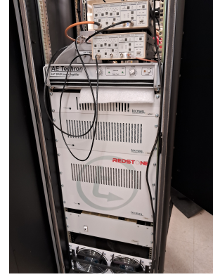
FIG. 6: Electronics cabinet, including the Redstone NMR system used to perform data acquisition and arbitrary waveform generation. The LVC2016 amplifier and SR560 pre-amplifier are at the top of the cabinet.
