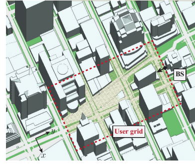
Fig. 2. The figure shows the adopted target scenario, which is built based on Times Square in Manhattan. The base station is positioned at a building, and the user grid is highlighted by the red box.
