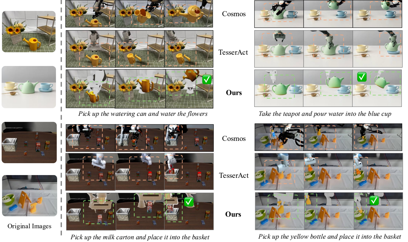
Figure 3. Qualitative comparison of robotic behavior generation using IGen. Given a single captured image and a natural-language manipulation instruction, Tesseract [76], Cosmos [2], and our IGen generate behavior observations. IGen produces more instruction-consistent and physically coherent object motions, closely matching the intended tasks. The green box represents action observations that adhere to physical laws and follow the task instructions, and the checkmark indicates task completion.
