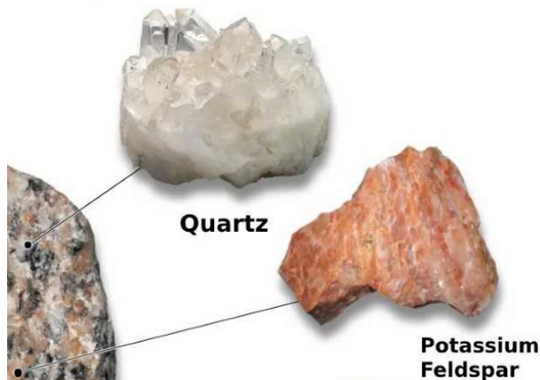
FIG. 3. Granite consist of several minerals but the largest fractions are quartz and feldspar. Our granite looks visually similar to granite whose composition has been studied in detail, with \approx 72\% quartz and \approx 15\% feldspar.
