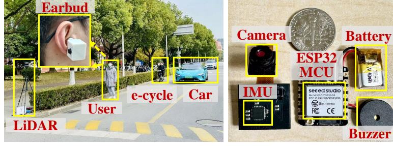
Fig. 5. The Prototype implementation of BlinkBud on an earbud (right) and an example of field study (left), where a volunteer wearing the earbud is walking along a road with motor traffic.
