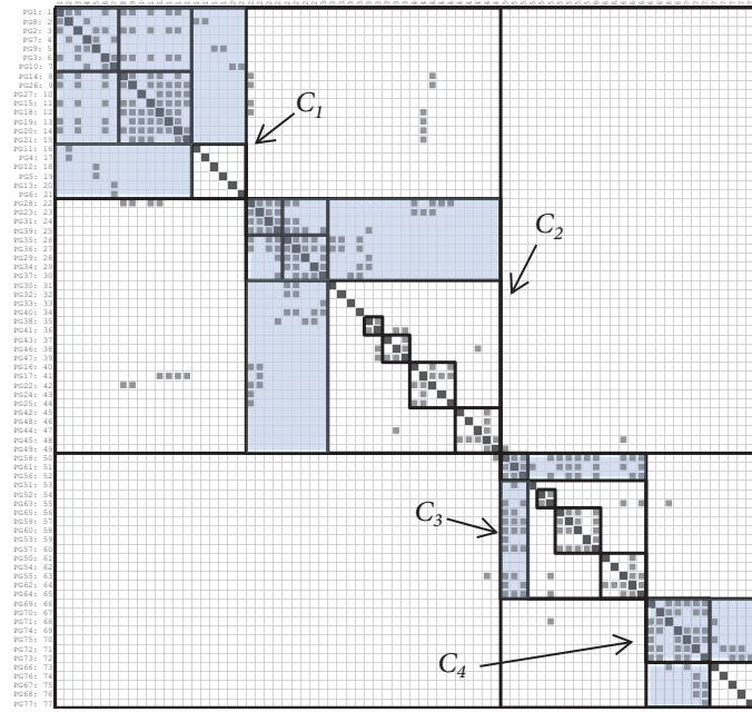
Fig. 7. The result of DSM-based clustering of the Festo with local buses. Bus detection is applied on clusters C_1 , C_2 , C_3 , and C_4 . The local bus for each cluster is highlighted in blue.
