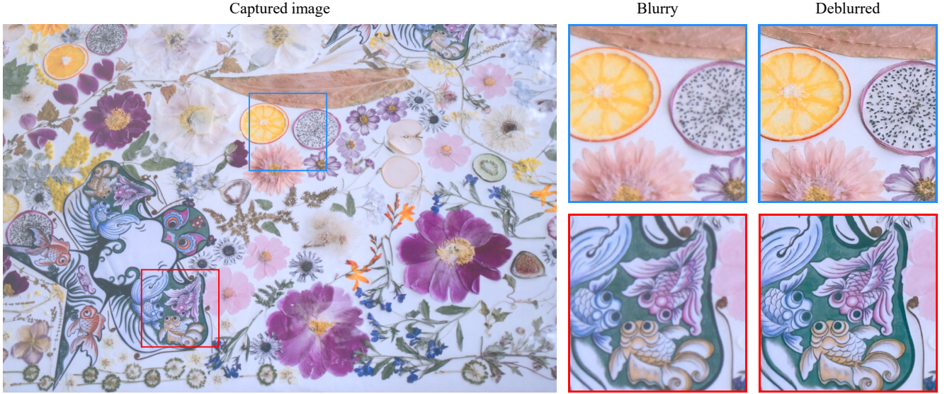
Figure 9. Deblurring results using PSFs estimated by CircleFlow. The left panel shows the captured blurred image, and the right panels display two representative regions before and after deblurring, where fine details are effectively restored.
