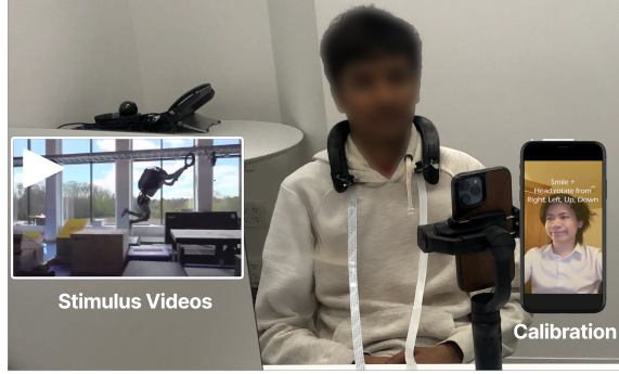
Figure 2: Study setup. In the Calibration round , the participant, wearing NeckFace [8], copies the movements seen on a video on an iPhone 11. The Stimulus round consists of a series of 30 videos played on a screen, while a webcam and NeckFace record facial reactions.
