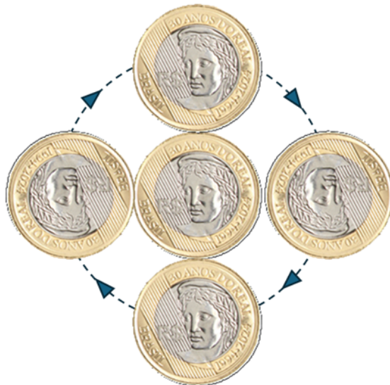
Figure 1: Illustration of the coin rotation paradox: a coin rolling externally around another identical coin completes two full rotations before returning to its initial position. The image shows a Brazilian one real coin (1 BRL).
