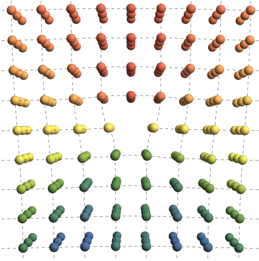
FIG. 1. Deformed crystal lattice in the presence of an edge dislocation. The rotation of crystallographic axes away from the dislocation core is apparent.
