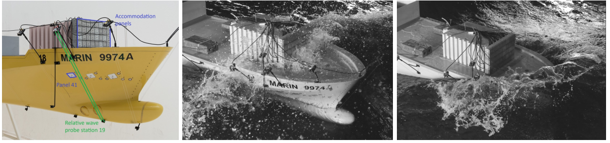
Figure 5: MARIN ferry 2 and the relevant instrumentation around the bow before the CRS SCREAM experiments (left), example green water impact (middle) and example bow-flare slamming impact (right).
