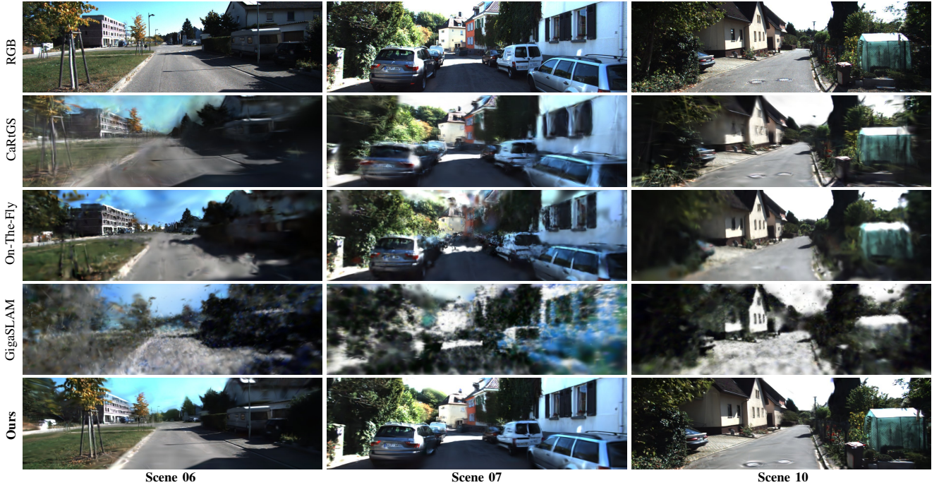
Fig. 3. Qualitative results on the KITTI [6] dataset. Reconstruction results on three scenes by all methods. On-The-Fly suffers from tracking drift and lacks loop closure. GigaSLAM’s neural approach fails without expensive post-processing. CaRtGS shows floating artifacts from missing depth supervision. Our method achieves superior quality through robust tracking, depth-supervised Gaussian placement, and efficient chunk-based optimization.
