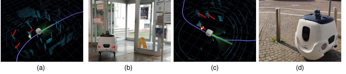
Fig. 15: Snapshots of autonomous navigation: exiting from building 1 through double automatic doors (a)(b) and passing through the bollards (c)(d). Pictures and screenshots are referred to the same location but not the same experiment.
