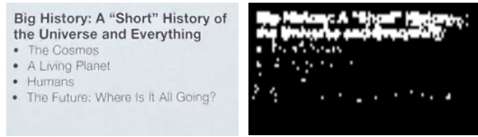
FIGURE 13. Examples of masking failures in SAEN model. An original image and mask image extracted by SAEN are shown on the left and right, respectively. For small-font characters, a heatmap becomes patch-like.
