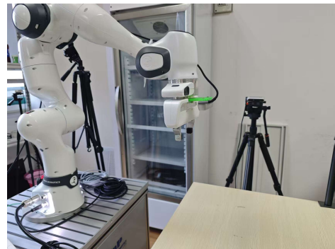
Figure 8. Real-world evaluation setup. Observations are captured using a side-view camera and a wrist-mounted camera, while an additional tripod-mounted camera records the scene from a rear-side perspective.
