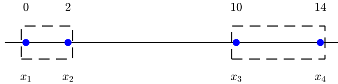
Figure 1. The original one-dimensional dataset X = [0, 2, 10, 14] to illustrate convex clustering and its robustness to data perturbations.
