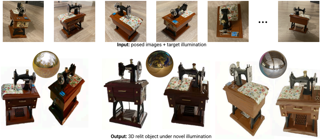
Figure 1: Given a set of posed images under unknown illumination (top), our method reconstructs a relightable neural radiance field (bottom), that can be rendered under any novel environment map without further optimization, on-the-fly relighting and novel view synthesis.
