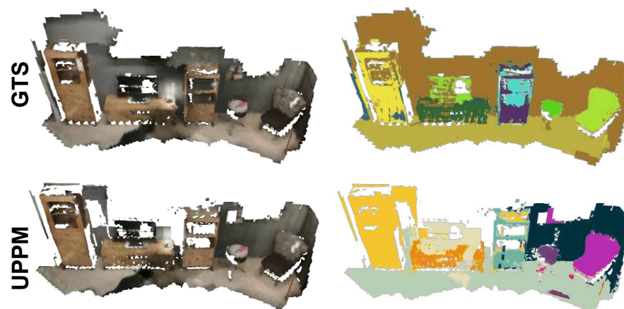
Figure 5. Qualitative comparison on the RIO dataset [62]. Top: Ground-truth panoptic segmentation and corresponding 3D map. Bottom: UPPM output with sharper object boundaries and more coherent semantic regions in cluttered, real-world scenes.
